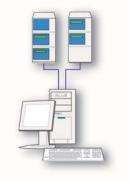
Data acquisition can also be performed with any detector providing a voltage output by simply connecting it to KNAUER IF2 or Smartline Manager 5000 A/D converter. ClarityChrom® allows to
