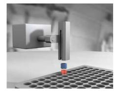
Mixing variables such as tumbling speed and duration can be programmed. Compared to the syringe aspirate/dispense actions offered by other autosamplers, mixing is much better and faster! Typical applications of this unique feature are internal standard addition, dilution, pre-column derivatization, homogenizing etc. Even in-vial liquid-liquid micro extraction is feasible.
